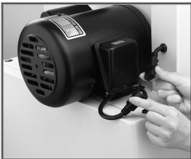
Figure 16. Plugging motor to switch.
